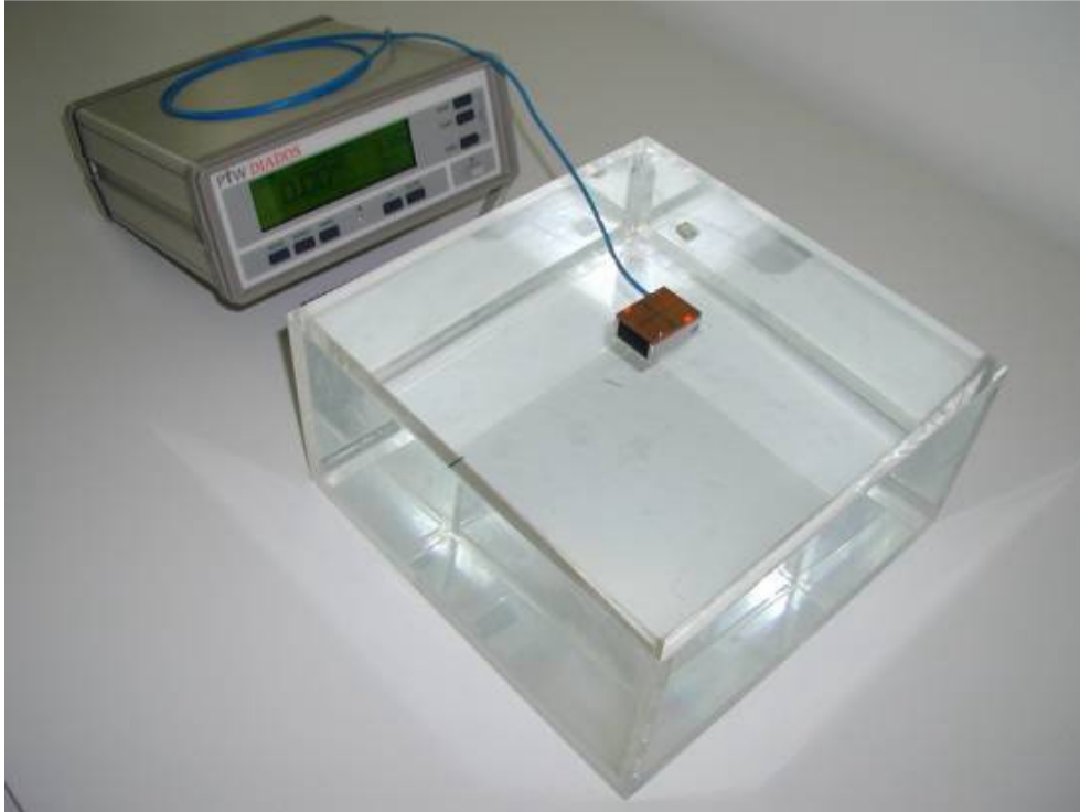
Fig.1: Circulating instrument of the ILC – IR4 with detector on the ISO water – slab phantom
